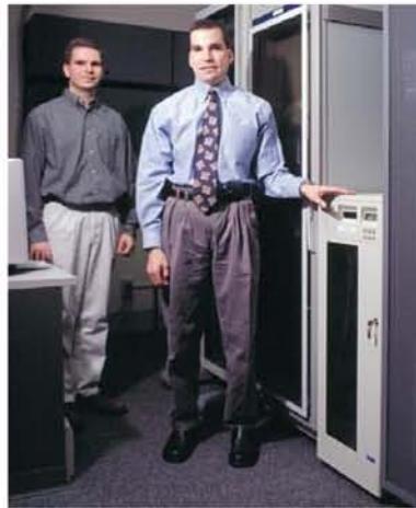
Bienia (left) and Hendricks (right) in the Clinic's Data Center. Qualstar's TLS-4660 Library equipped with AIT-2 drives and 63 tape slots can handle 3.15 terabytes of data. The performance verdict from Bienia: "Flawless. We've been live in production since August, we've had zero trouble."
